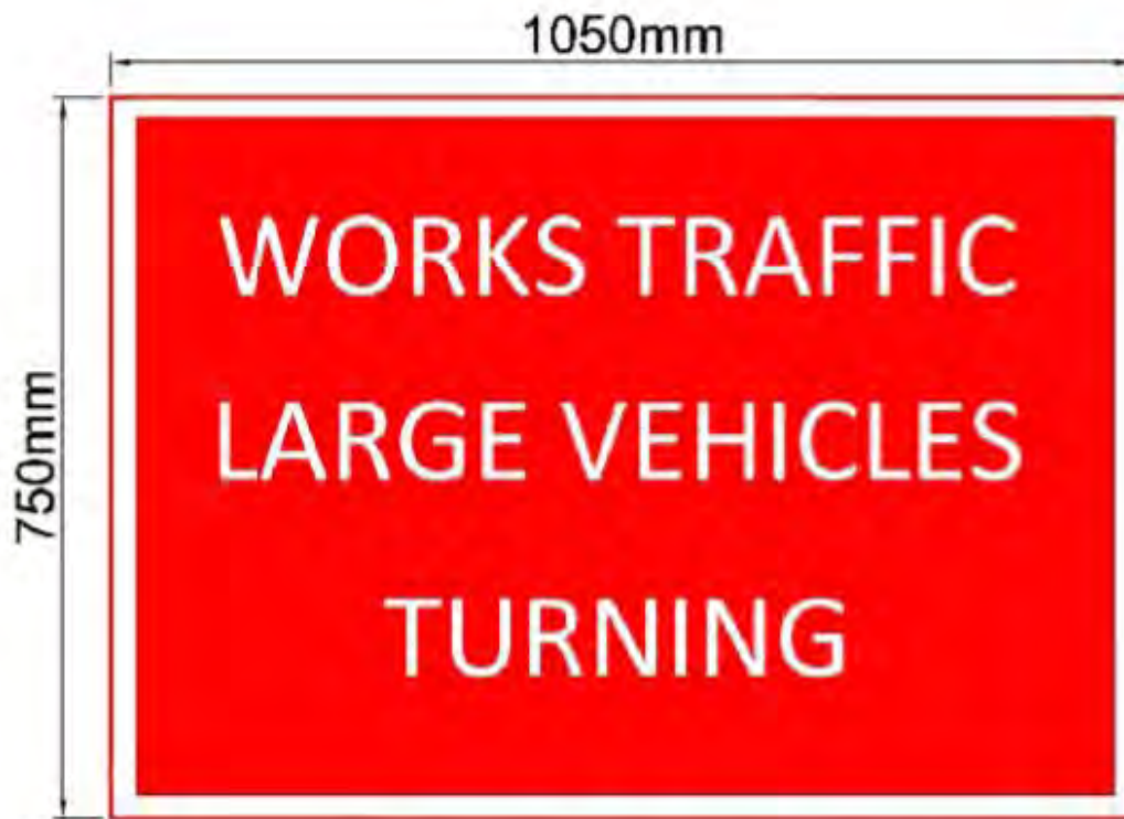
1. Temporary Construction Traffic signage (Diagram 7301 'WORKS TRAFFIC' in the TSRGD)
